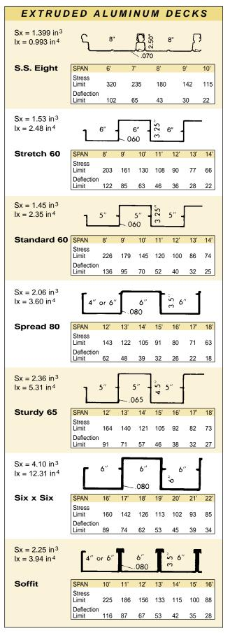
Tables show allowable loads (lbs. per sq. ft.) All extrusions are 6063-T6. Safety factor of 2.1 Yield: 31,000 psi. Figures based on breaking deck at alternate bends.
